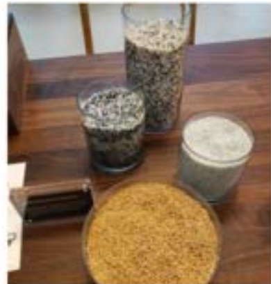
The resin pellets used to create the 3D printed pieces is made from leftover food waste.
